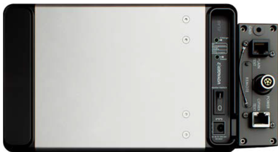
Voyager 2 rear showing UBI-2590 battery, DC input and HAIPE power
